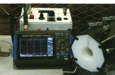
The controller is equipped with an analog output terminal (BNC terminal). Connect a recorder, oscilloscope, or the like (optional) to the terminal for confirmation of data on the spot.
